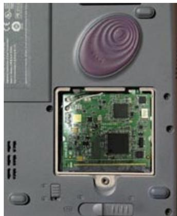
*The Mini PCI slot supports "hot swapping" of Mini PCI adapter, allowing you to insert or remove the ParkerVision miniPCI1500 Wireless PC LAN Card from the slot whenever you like, even when power to your computer is on. However, you should always disable the ParkerVision miniPCI1500 Wireless PC LAN Card prior to card removal to allow Windows to log off from the network server.*
