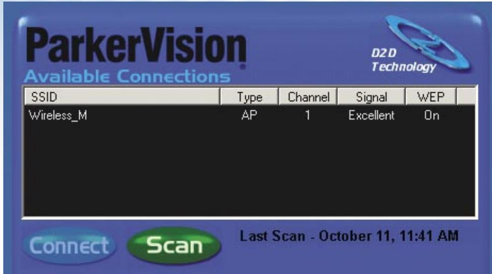
The top-most section of the D2D Configuration Dialog Box shows the available connections. The available connections will be displayed from a scan performed when the software was started, or when the scan button was clicked.
